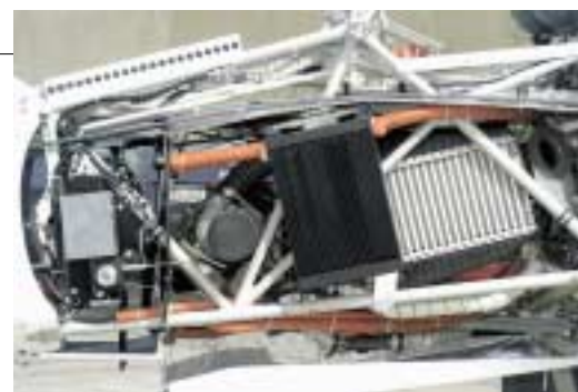
Turbo-oil cooler - intercooler (from left to right)
