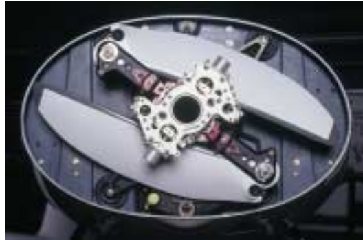
STEMME RETRAC propeller folded
