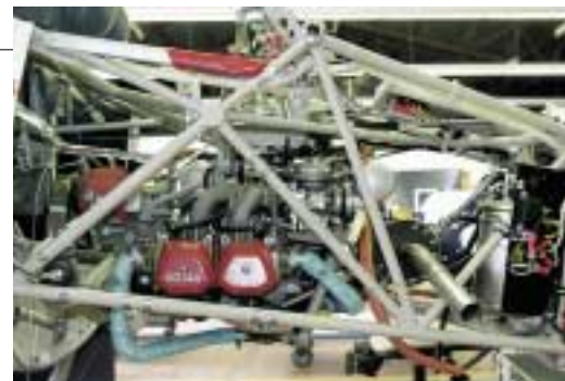
Engine without cooler and firewall
