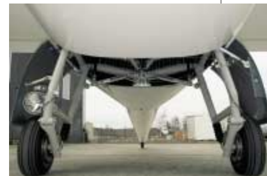
An unconventional gear, to be folded into a minimized fuselage cross section.
