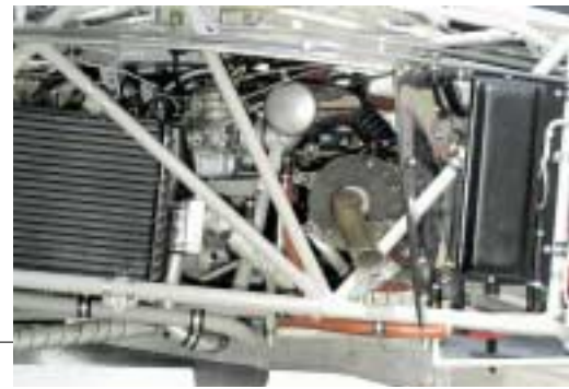
High precision mixer and control push rods to ailerons, flaps & airbrake
