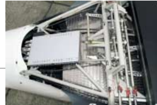
High precision mixer and control push rods to ailerons, flaps & airbrake
